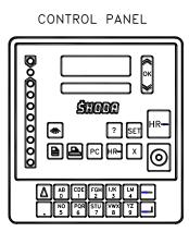
Hardness tester RB-1E is recommended for material hardness tests, where either the Rockwell C, B, A, D or F method according to ČSN EN 101109 or the Brinell (ČSN EN 10003) method can by selected. Hardness tester RB-1E includes an electronic control unit providing for the following functions:
